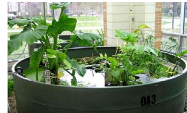
The above image is an aerobic reactor at Oberlin College's Living Machine™
